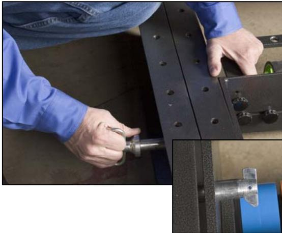
Find the safety pin in each side rail. They are located between the cable sorter and the tape shaft.
