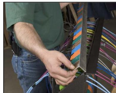
Lift the uppermost fin from the labeling spindle (*middle*) and insert it in the slot along the top of the head (*right*), making sure that the cutout midway along the fin fits around the clamp.
