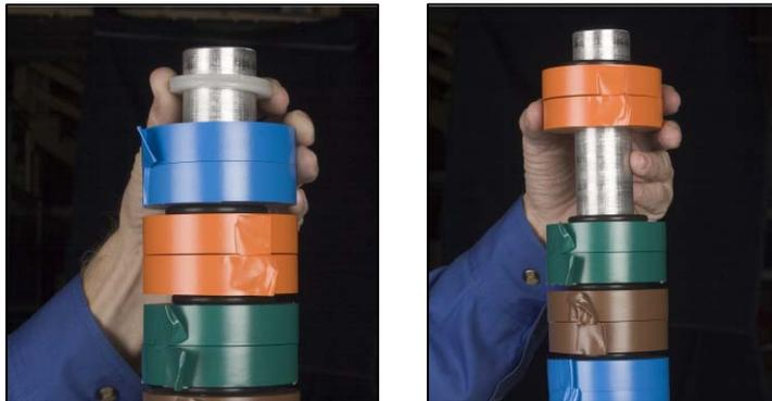
To reload the shaft, alternatively slip a roll of tape and a plastic washer onto the tape shaft. Remember, to load the tape rolls in the proper color sequence (i.e. two rolls of the same color followed by two more rolls of identical color)
