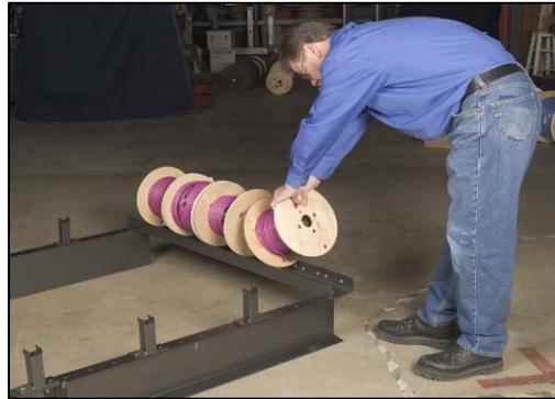
**Tip:** Place reels on the staging channel so that cable feeds over the tops of reels. This helps to reduce the bend radius of the cable as it is fed into the sorter.
