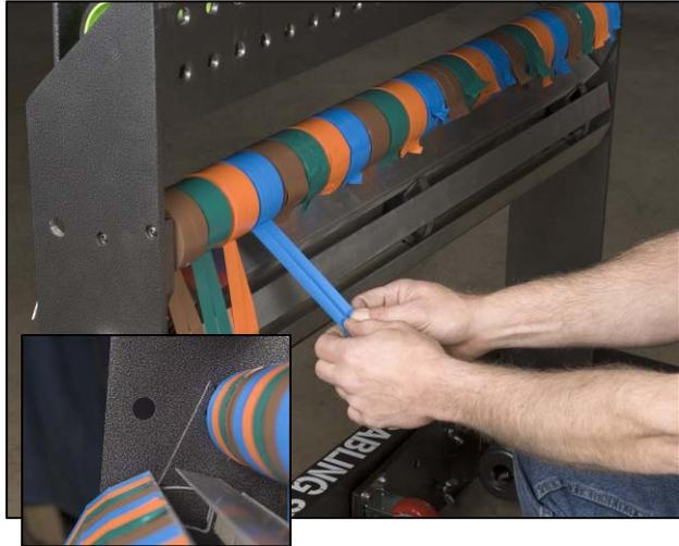
**Tip:** Pulling the tape stretches it. Let the tape relax before sticking it to the labeling fins.
