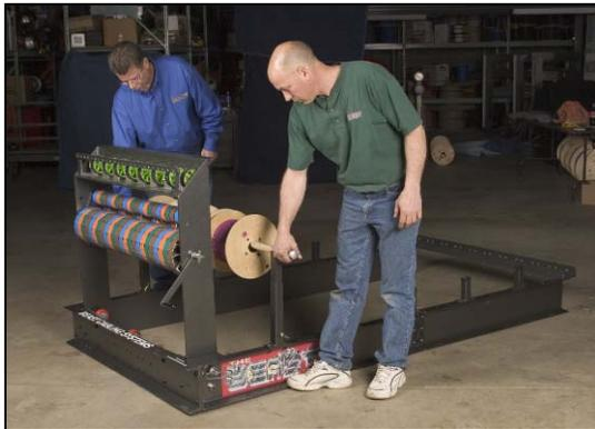
With a helper, lift the reels from the staging channel onto a pair of the stanchions that you installed earlier (*left*).
