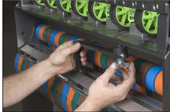
Return cable reels to the staging channel, extract the pole, and set the reels aside.
