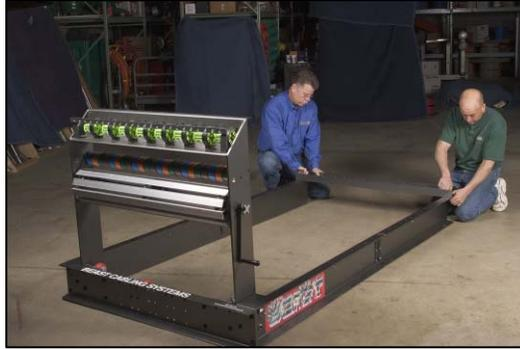
**Tip:** Mounting the staging channel with its holes toward the rear leaves additional side-rail holes available for stanchions.
