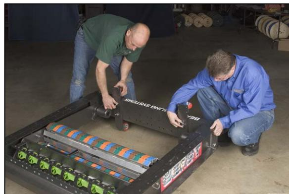
**Tip:** To support the Beast I/II while you reinstall the wheels, slip a scrap of two-by-four under the base.
