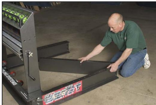
Place the staging channel on top of the side rails, and secure it with the bolts and wing nuts.
