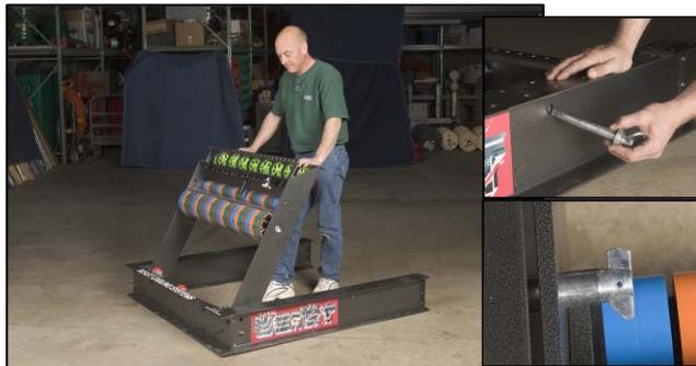
**Caution:** Keep hands and feet clear of the side rails as you lower the head. Although the head is counterweighted with springs to keep it from falling, there is risk of injury if the head is lowered on a hand or foot.
