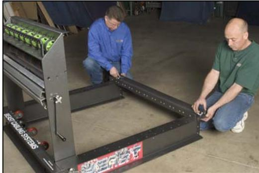
Unfold the left and right side rails one at a time.
