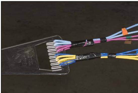
Fold cables into the comb at the wide end of The Claw, placing the cables for each drop next to each other—or on top of each other in the same comb space. Each can hold four cables.
