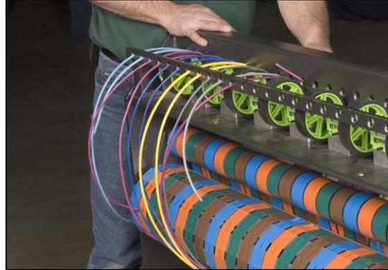
**Tip:** To thread additional cables, remove cable counters and thread each cable through only one guide bar.
