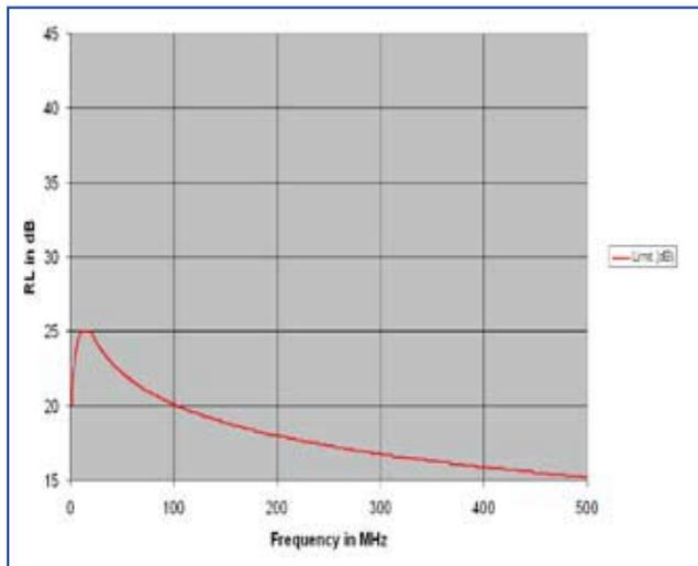
FIGURE 2: Current return loss limit for category 6A cable
