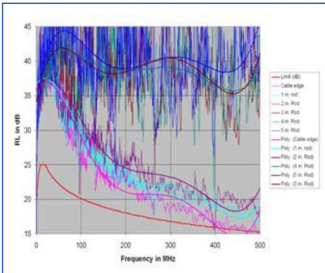
**FIGURE 3:** Return loss results using static rods
