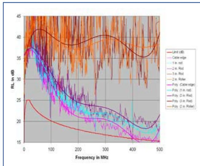
**FIGURE 4:** Return loss results using static rods and 2-inch roller
